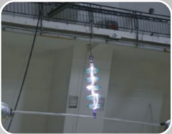
工频湿耐受电压试验 Wet power-frequency voltage test
