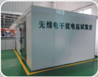
无线电干扰电压试验 Radio interference voltage (RIV) test
